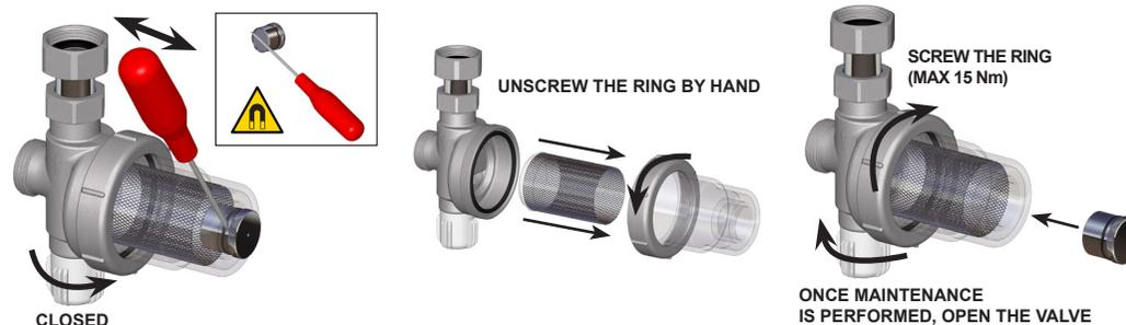
1- Close the valve. Remove the magnetic insert from the socket with the aid of a screwdriver
